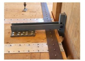
Left: Out-of-plane brace for the wall; Right: Complete wall-to-floor connection with shear key in the middle and braces on either side.
